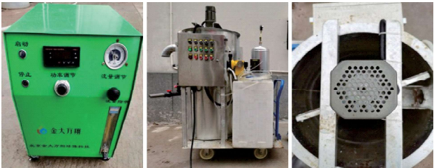
图2 臭氧气浮装置 Fig.2 The dissolved ozone flotation system
