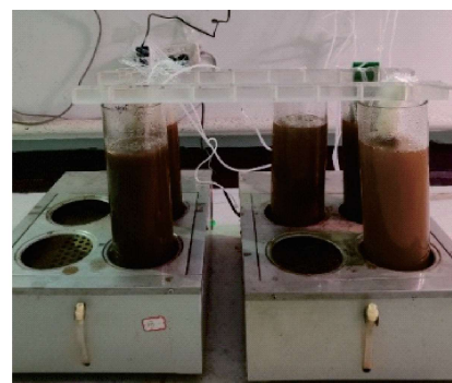
图2 人工水草组合微生物菌剂反应器 Fig.2 Reactor of artificial aquatic weed combined microbial agent
